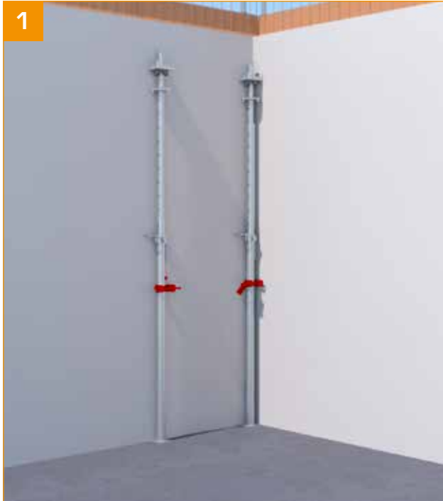
- Position and clamp the first two props. → Here, using the HorizontalAL steel prop clamp.
